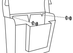
2. Remove inner basket. Place receptacle on bottom screw. Install top screws. Replace inner basket.
